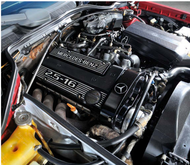
Above: 16v motor derived from M102 four-cylinder.
